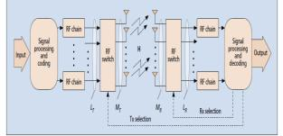
Figure 1: Antenna selection in MIMO system
