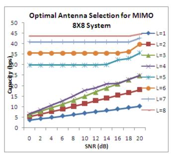
Figure 2: capacity of optimal Antenna selection for 8X8 MIMO system Table 1: Capacity values of optimal Antenna selection in 8X8 MIMO for different antenna selection Factor L as a function of SNR
